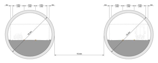
**DOUBLE-BORE**15.4M (50 feet) Bore with 3 Traffic Lanes per Tunnel
